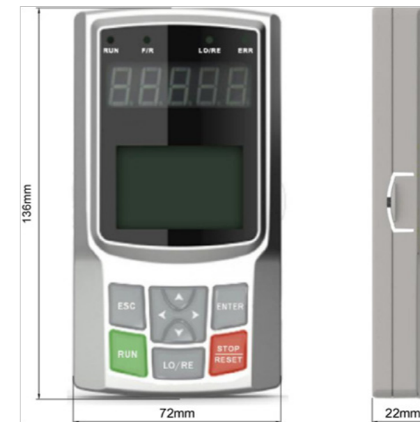
Fig. a Dimensions of standard LED keypad for AS180N inverter (supporting installation on cabinet door)
