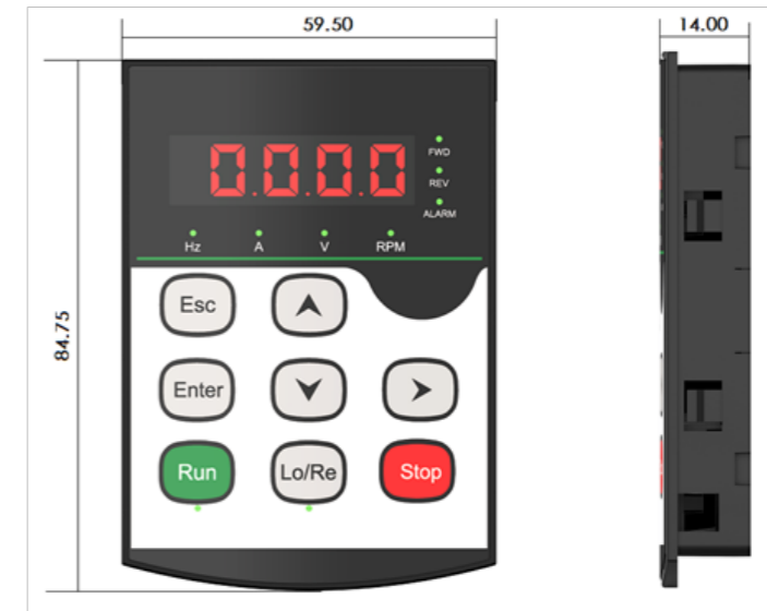
Fig. a Dimensions of standard LED keypad for AS180N inverter (supporting installation on cabinet door)
