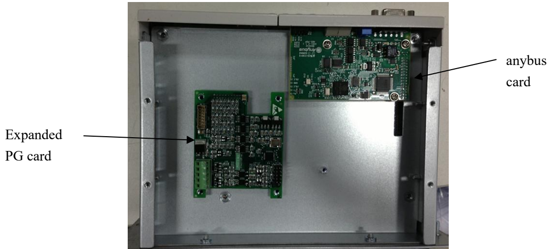
Figure 4-14 Insertion position diagram of anybus card and expanded PG card
