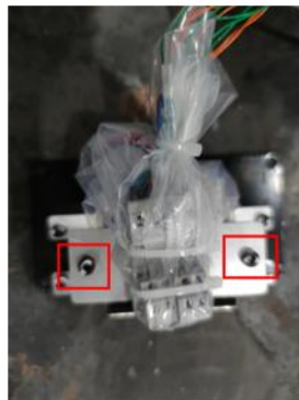
Figure 2.10 Schematic diagram of the positions of the two fixing screws
