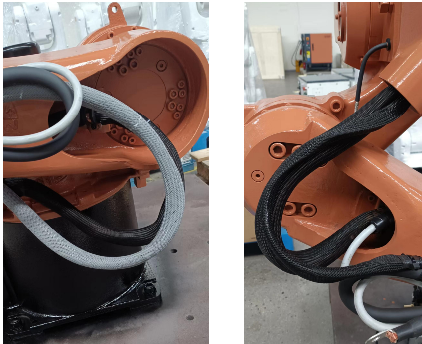
Figure 2.1 Main cable protection inspection
