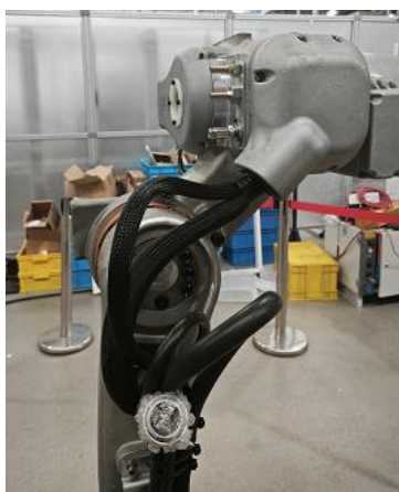
Figure 2.1 Main cable protection inspection
