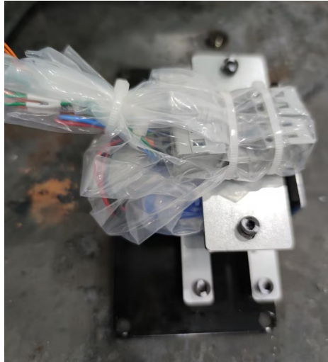
Figure 2.13 Cable tie fixing diagram
